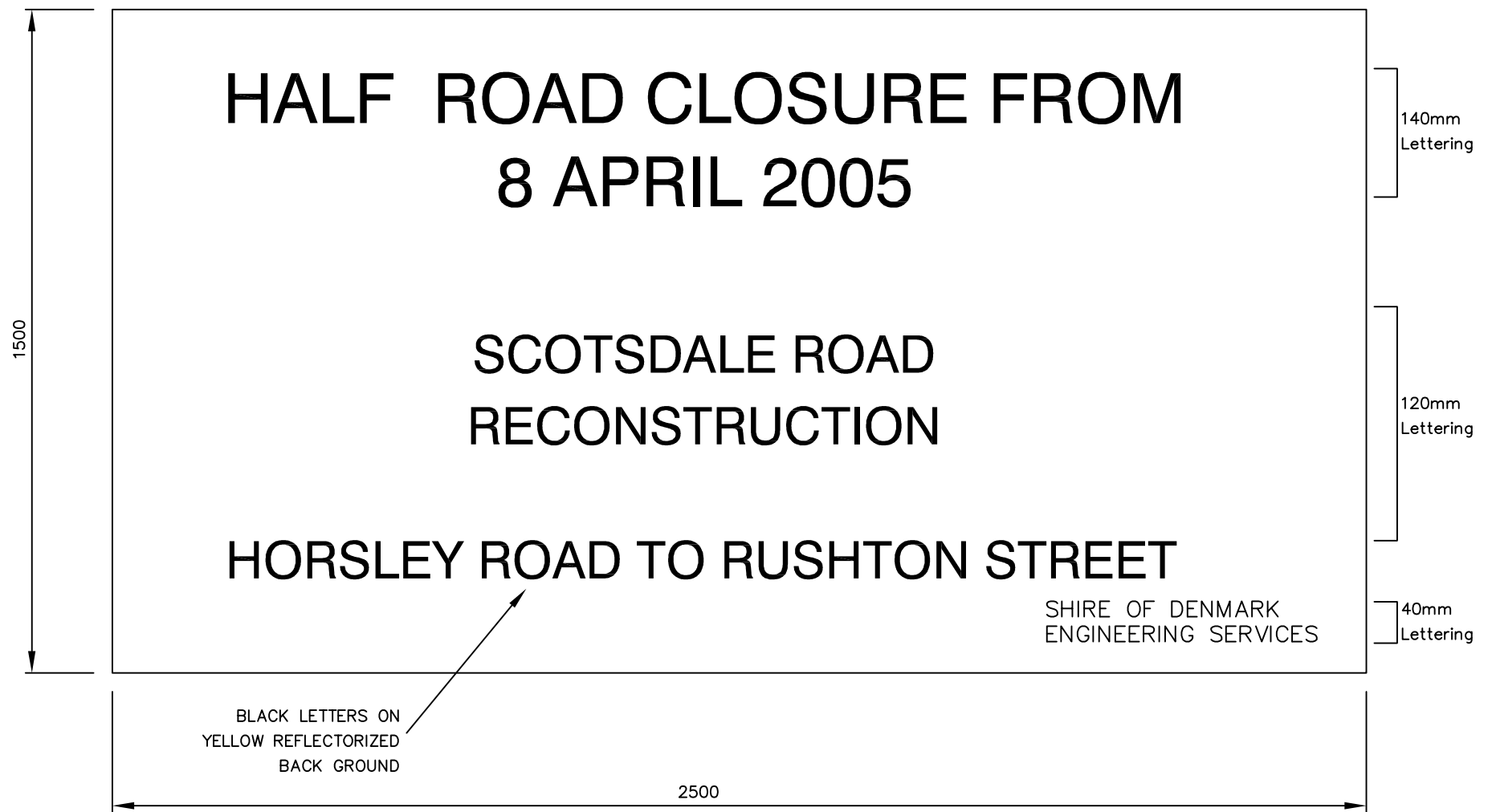
WORKS INFORMATION SIGN
