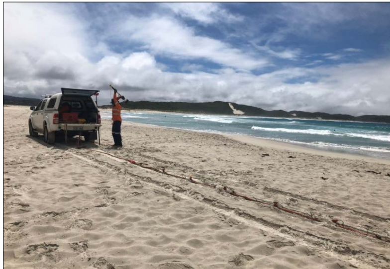
Figure 5: MASW data acquisition along Ocean Beach.
