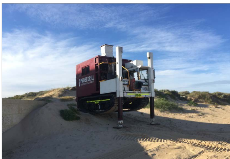
Figure 6: CPT carried out during a previous coastal investigation by GBGMAPS.
