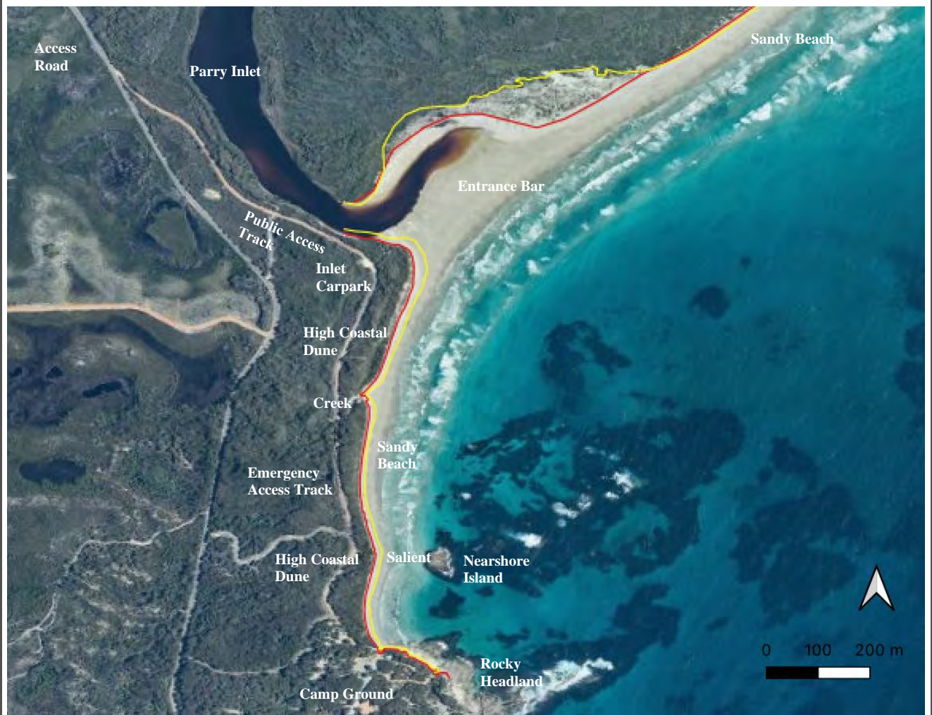
Parry Beach 2021 imagery showing key geomorphic features and Shire assets. Note 2001 coastal vegetation line shown in yellow, and 2021 coastal vegetation line shown in red.
