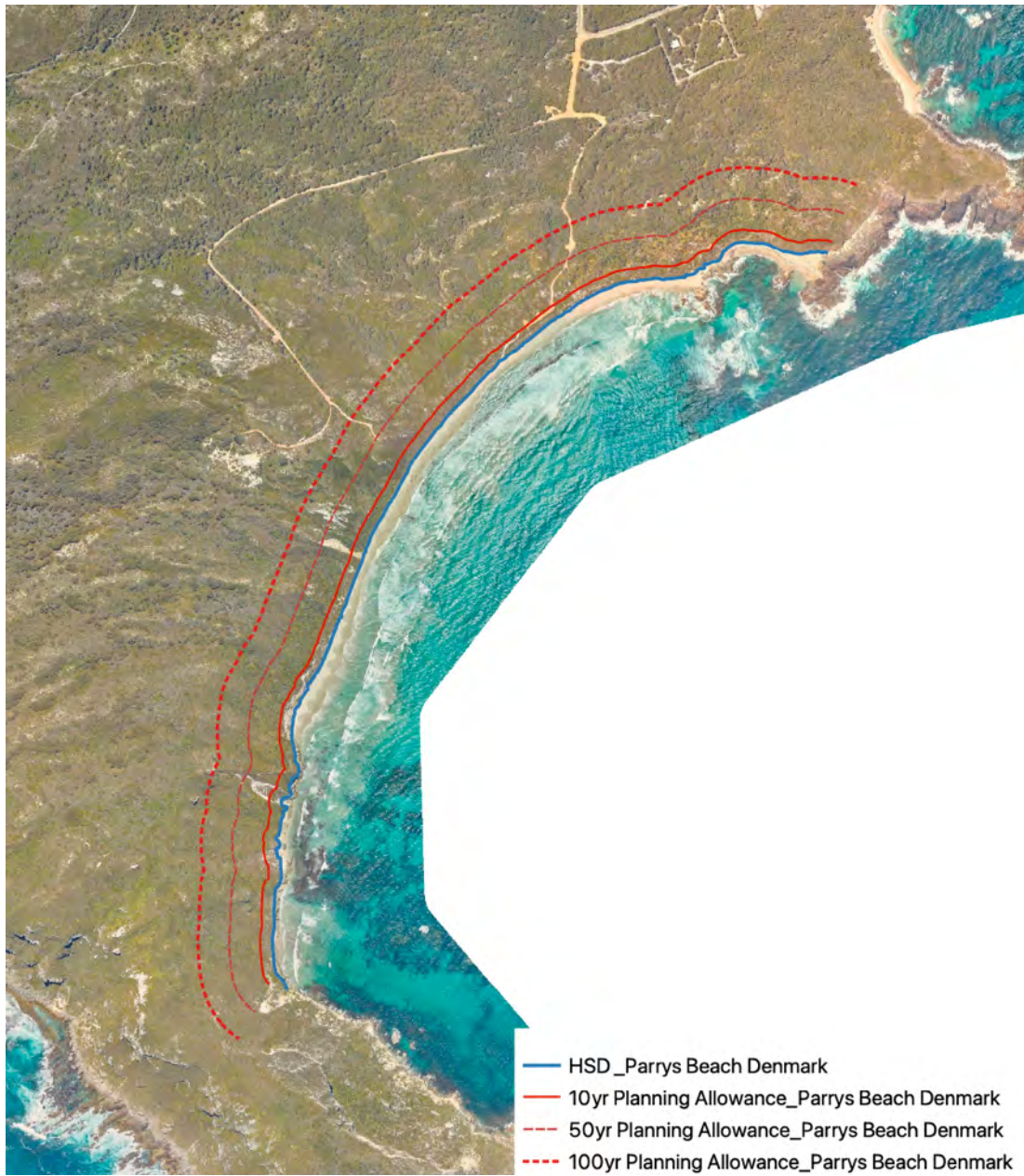
Figure 6-2 Mapping of planning allowances for coastal areas at Parrys Beach Reserve (Hillier)
