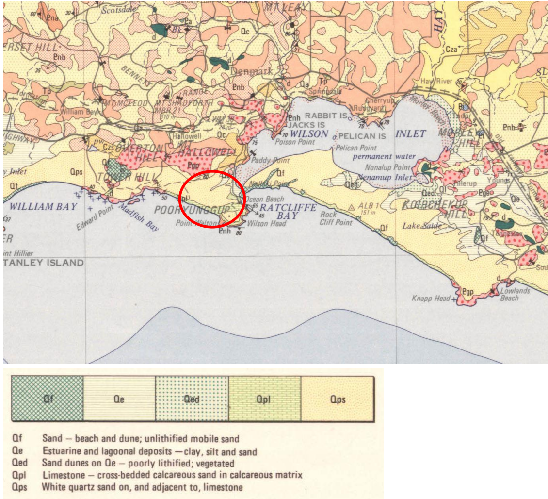
Figure 3: Site Geology – Ocean Beach Lime Quarry ( http://www.geoscience.gov.au )
